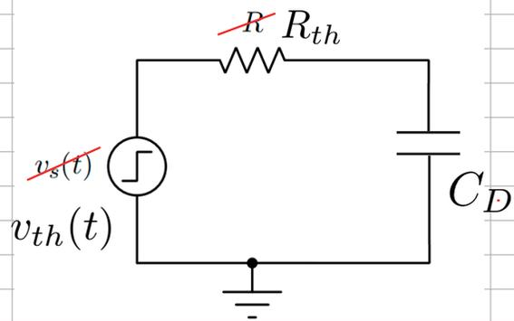
$$v_d(t) = \Delta V \left( 1 - \exp\left(-\frac{(t - t_0)}{RC}\right) \right)$$
