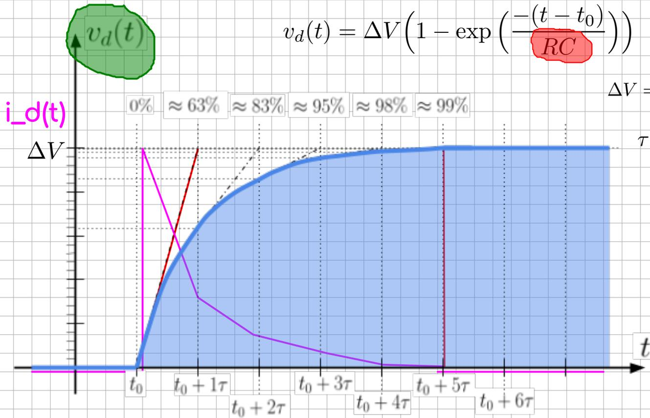
$$v_d(t) = V_F + (V_0 - V_F) \exp\left(-\frac{(t - t_0)}{RC}\right)$$
